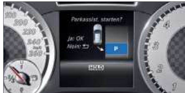
The display in the instrument cluster gives you a clear picture of what is happening during the current parking process.
