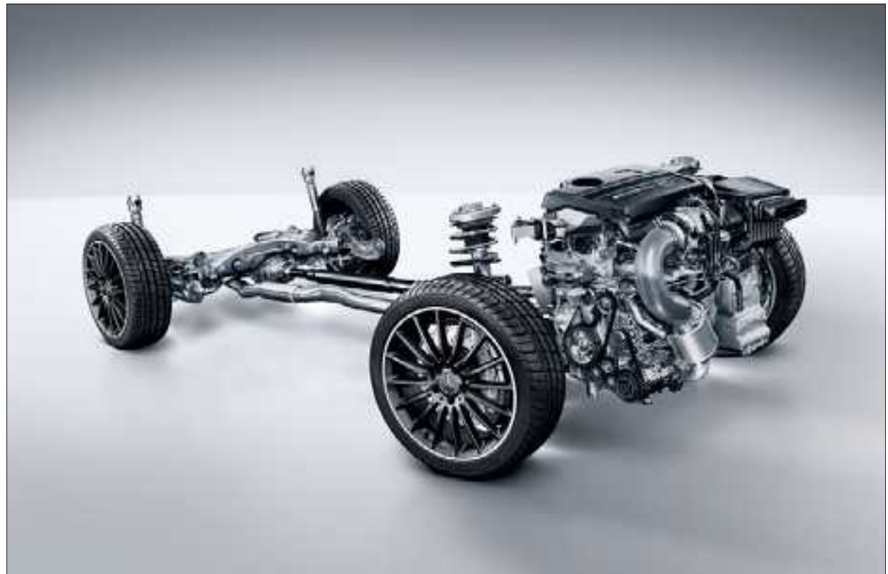
Autonomous steering knuckles at the front with AMG-specific elastokinematics increase dynamism through stiffer axle bearings.
