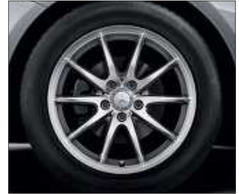
10-spoke light-alloy wheels with 225/45 R 17 tyres (optional, standard for B 250), Code R43.
