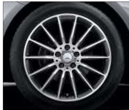
AMG multi-spoke light-alloy wheels, painted titanium grey with a high-sheen finish, with 225/40 R 18 tyres, Code 791.
