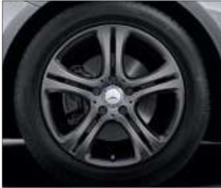
5-twin-spoke light-alloy wheels, painted tremolite grey, with 225/45 R 17 tyres (optional), Code 44R.
