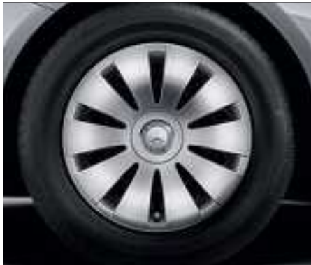
Steel wheel with 10-hole wheel trim with 205/55 R 16 tyres (standard for B 200 CDI, B 220 CDI, B 200 and B 220 4MATIC), Code 643.
