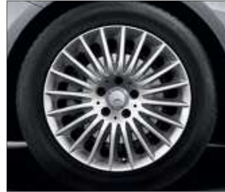
Multi-spoke light-alloy wheels with 225/55 R 17 tyres (only for B 200 Natural Gas Drive), Code 08R.
