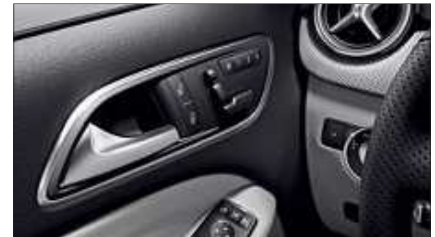
The electric seat adjustment with memory function remembers up to three individual settings.
