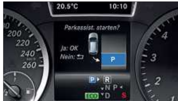
The display in the instrument cluster gives you a clear picture of what is happening during the current parking manoeuvre.
