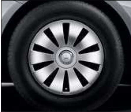
Steel wheels with 10-hole wheel trim with 195/65 R 15 tyres (standard for B 160 CDI, B 180 CDI, B 180 CDI BlueEFFICIENCY Edition and B 180), Code R00.
