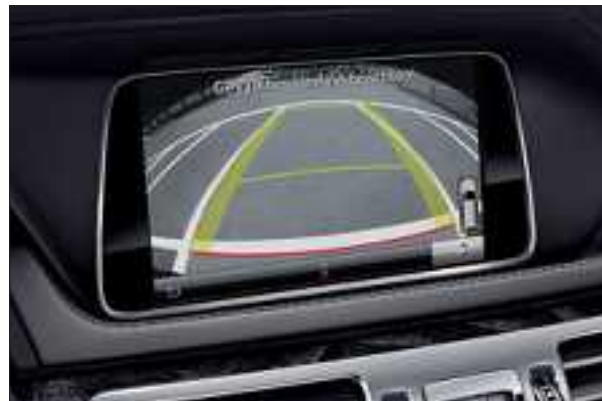
During parking, the COMAND Online central display shows the area behind the car
