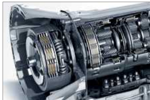
The AMG SPEEDSHIFT MCT 7-speed sports transmission
