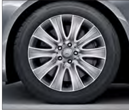
10-spoke alloy wheel with 245/50 R 18 tyre (code R41).
