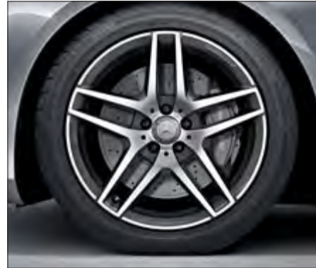
AMG 5-twin-spoke high-sheen alloy wheel finished in titanium grey, with 245/45 R 19 front tyre and 275/40 R 19 tyre for the rear (standard for AMG Line, code 793).
