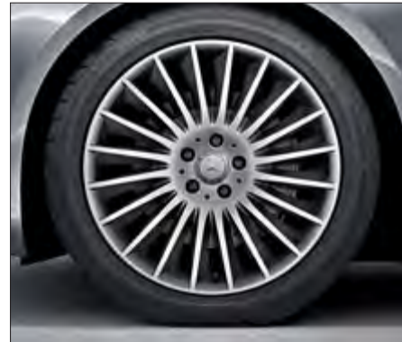
Multi-spoke alloy wheel with 245/45 R 19 front tyre and 275/40 R 19 tyre for the rear (code 11R).
