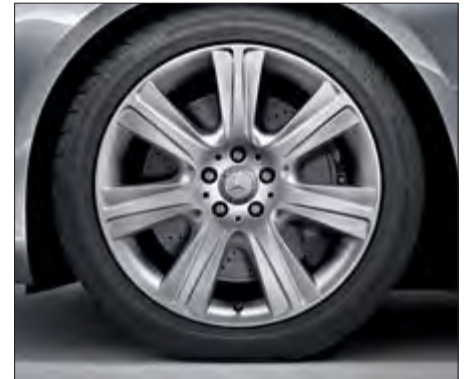
7-triple-spoke alloy wheel with 245/45 R 19 front tyre and 275/40 R 19 tyre for the rear (code 12R).
