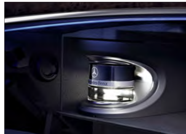
AIR-BALANCE package, including ionisation, air filtering and fragrance.
