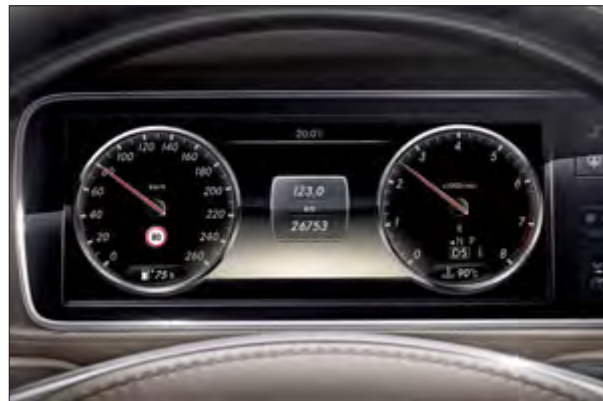
Traffic Sign Assist can recognise speed limit signs and show the speed limit in the display.
