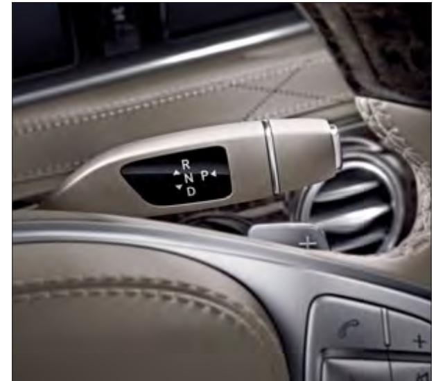
DIRECT SELECT lever on steering column. The driver can also change up or down a gear manually using the additional shift paddle.
