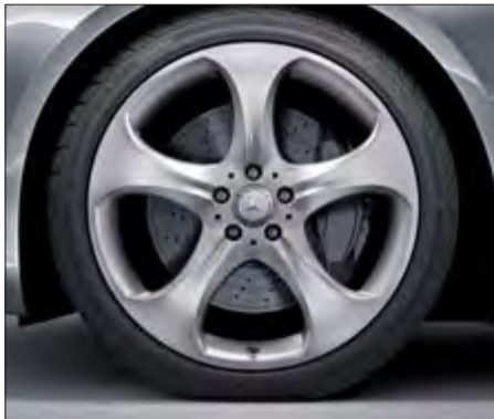
5-spoke alloy wheel with 245/40 R 20 front tyre and 275/35 R 20 tyre for the rear (ex-factory accessory wheel, code 53R).
