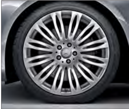
Multi-spoke alloy wheel with 245/40 R 20 front tyre and 275/35 R 20 tyre for the rear (code 13R).
