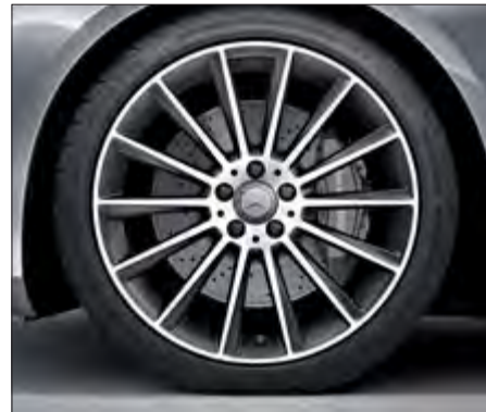
AMG multi-spoke high-sheen alloy wheel finished in titanium grey, with 245/40 R 20 front tyre and 275/35 R 20 tyre for the rear (code 769).
