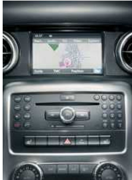
Standard equipment. TFT colour display with 17.8 cm screen diagonal for displaying high-resolution maps.
