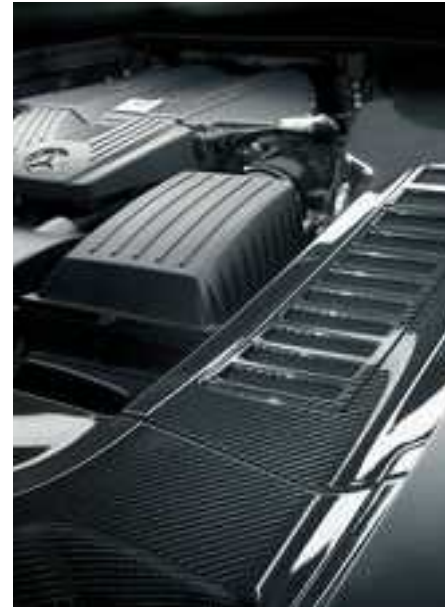
AMG carbon-fibre engine compartment cover.
