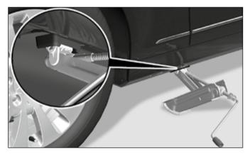
The positioning points for the vehicle jack, using the C-Class as an example (just in front of or behind the relevant wheel arch). The specific jacking points for the model in question are shown in the owner's manual.
